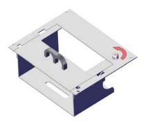
Turn knob to tighten and secure the two faceplate pieces together.
