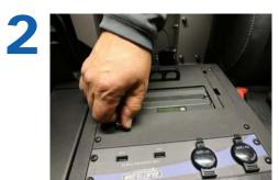
Loosen knob to release the printer faceplate from its secure position.
