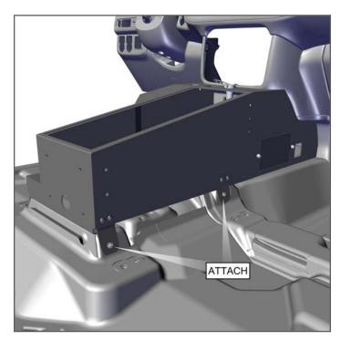
Adjust Mounting Legs as needed - to position over OEM mounting points and tighten legs to Contour Console. Secure Mounting Legs to OEM Substructure using OEM 12MM bolts or provided 1/2" - 13 x 1.5 TCS Bolts.
