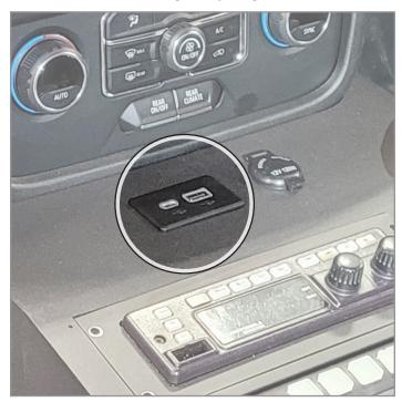
Relocate OEM USB/Line-in housing to Contour Console and re-connect previously removed cables.
