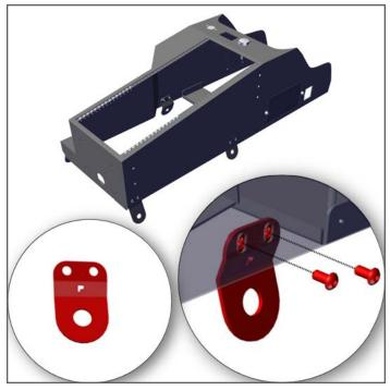
Outside of vehicle, loosely attach Rear Legs, Front P/S, and Front D/S Legs with provided hardware. Install Contour Console into the vehicle from the rear seat area, sliding forward until mating up with OEM dash structure.
