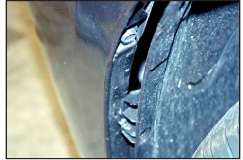
Remove 4 retainer clips from plastic wheel well liner. Pull liner away to expose 2 - 10 mm bolts per side.
