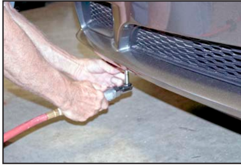
Remove 6 screws using a 7 mm socket from the underside of OEM bumper.
