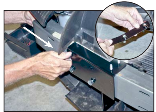
Using provided installation tool, slide backing plate onto tool. Then proceed to insert backing plate/tool into bumper frame. Position brackets center most in the slots they go into. Line up with holes on mounting bracket. Secure with (4 ea.) 1" hex head bolts per side.
