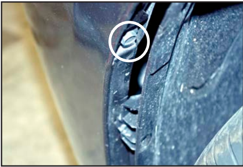
Remove 4 - 10 mm bolts per side from lower air duct on inside of wheel.
