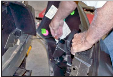
Pull OEM bumper away and unplug lights.
