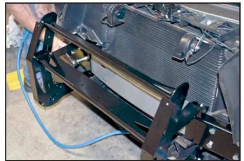
To test the proper alignment of the brackets, temporarily install the universal vertical bumper assembly. Once confirmed, tighten all brackets and remove the universal vertical bumper assembly. Now reinstall OEM bumper by reversing steps 1-5 of these instructions.
