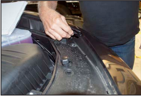
Remove 12 plastic retainer clips and 2-10mm bolts from top of OEM bumper.
