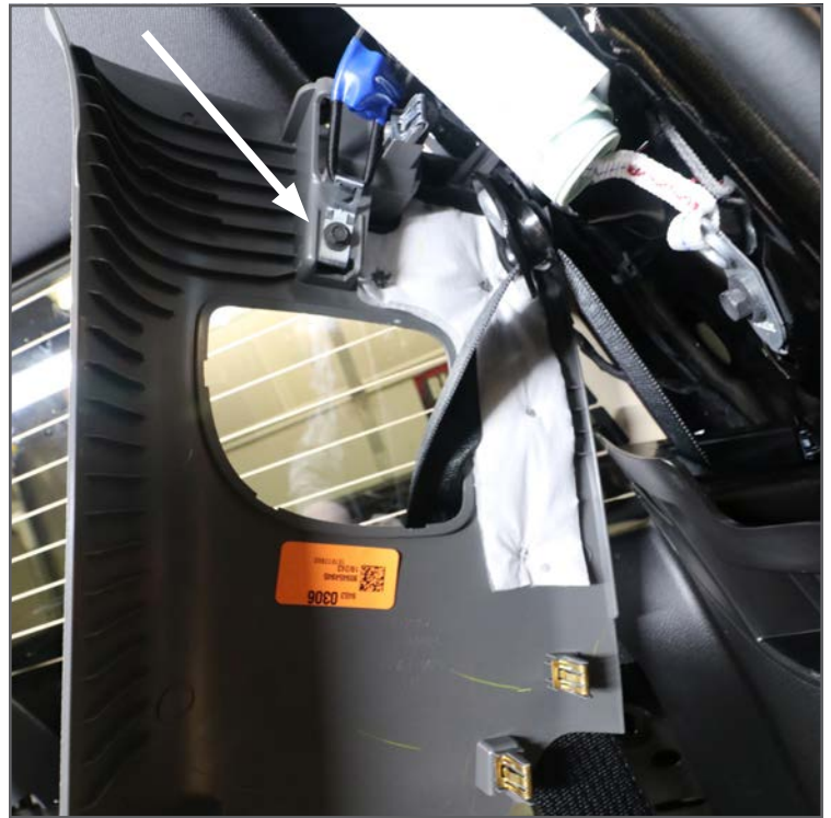
5. Remove the 7 mm screw attaching trim to the vehicle via nylon strap.
