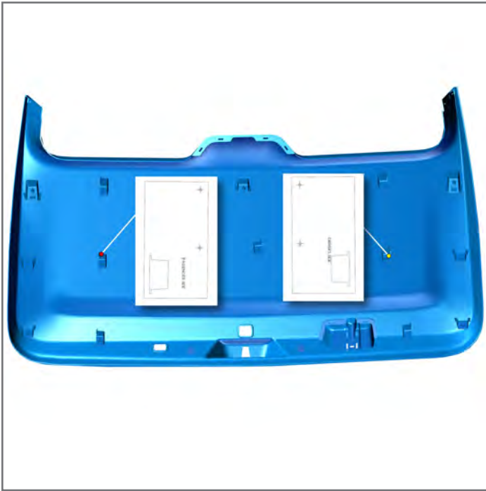
3. Cut out provided templates and set over standoffs of the DS/PS plastic trim. Mark and drill (2) 1/16 holes per side as indicated on template.
