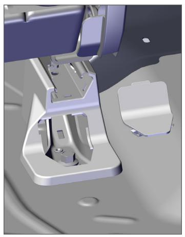
1. Remove cap from inside back seat rails of front seats. Remove (2) 13mm seat bolts nearest the console.
