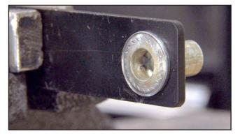
7. This will allow the AVK Fastener to secure onto the backside of the metal.
