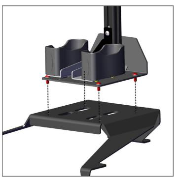
Reposition mounting plate under the seat rails and tighten all OEM seat bolts, replace trim cover and use provided hardware for AVK locations.
