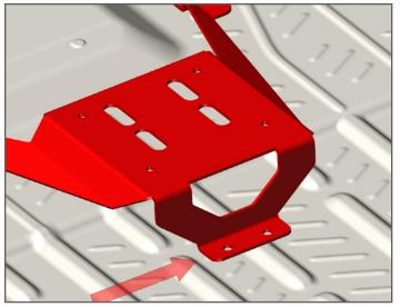
2. Slide GR6 mounting plate under the inside seat rails of front seats. Mark hole location for rear of mounting plate for AVK install. Remove mounting plate and set aside.
