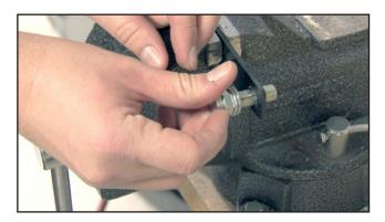
Place into 1/2" drilled hole.
