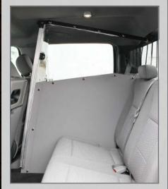
The upper 1/3 is polycarbonate and has been designed to allow for prisoner viewing/interaction but not diminish drivers view out the rear view mirror. In fact, the visibility for an officer is nothing short of amazing.
