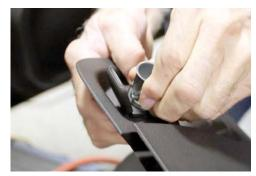
Remove OEM 12V outlet from minicompartment and relocate into Jotto Desk console.
