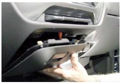
Pull mini-compartment away from OEM dash releasing clips.
