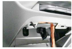
Insert bolt spacer/stud into slots into where clips on OEM mini-compartment.
