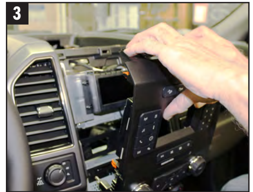
3. Pry from the top to unsnap the trim covering the radio and climate controls. Unplug the heater control from the harness.
