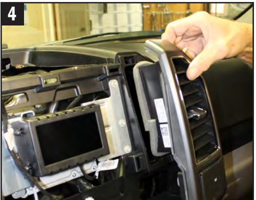
4. Remove the left and right climate sections containing the 12"volt plug and the 4x4 knob selector, unplugging each from the wiring harness.
