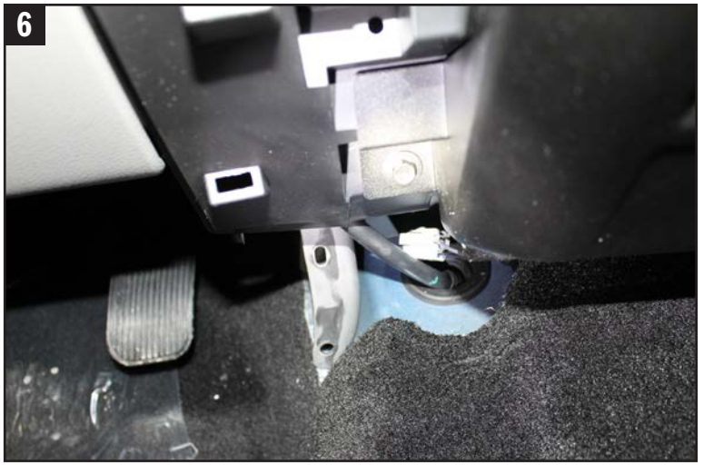
6. Remove lower panel containing 12 volt power and USB by unscrewing (2) 7 mm screws on the top and (2) 10 mm screws on the bottom. Unplug accessories from harness.
