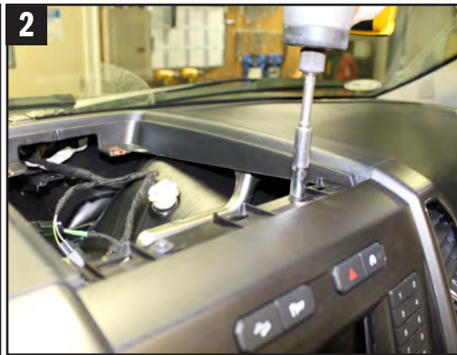
2. Pry the top tray up from each front corner and remove the (2) 7 mm screws. Unplug speaker from the harness.
