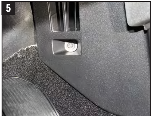
5. Remove (1) 10 mm screw holding the lower trim in place rotate over the transmission hump and unsnap from the passenger side.
