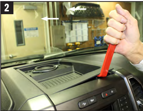
2. Pry the top tray up from each front corner and remove the (2) 7 mm screws. Unplug speaker from the harness.
