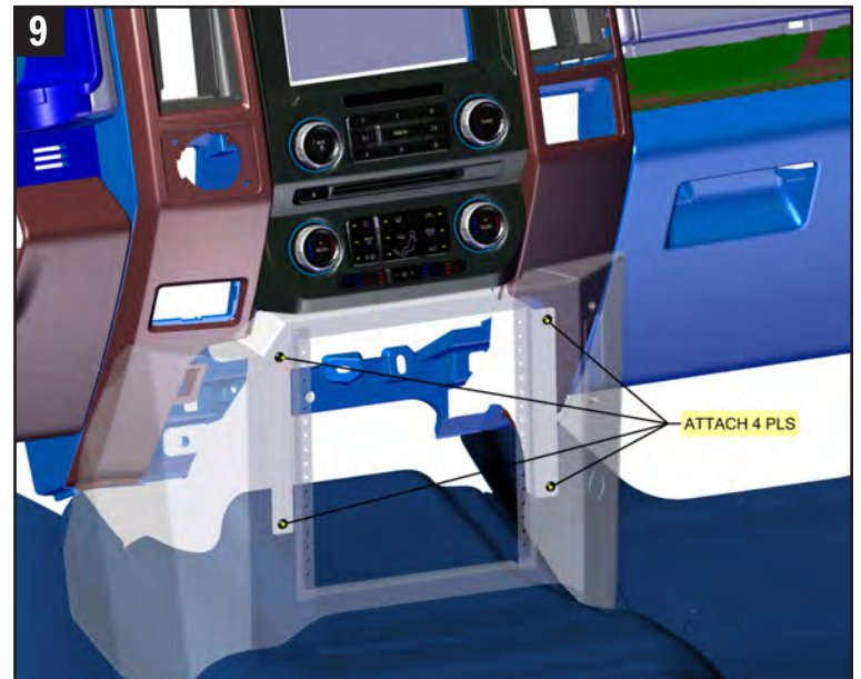
9. Attach the Console to the Console Support Bracket with provided hardware.
