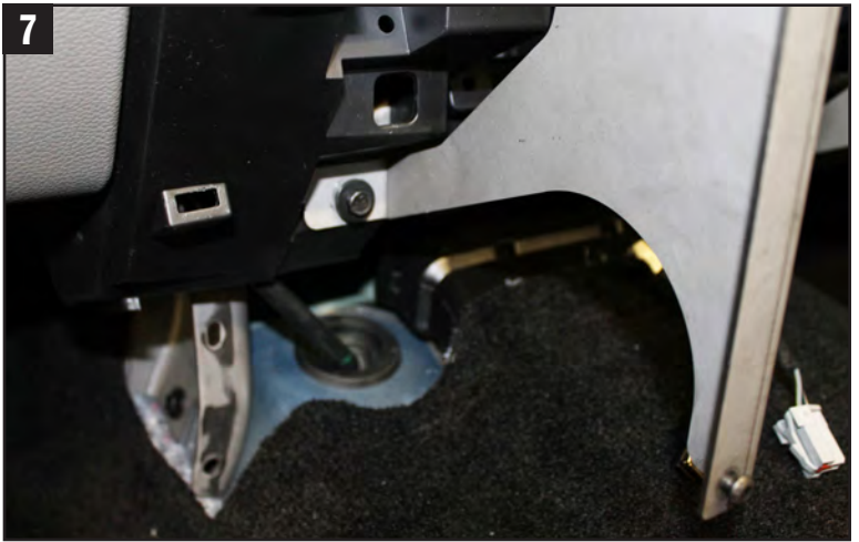
7. Install the Console Support Bracket with the previously removed 7 mm and 10 mm OEM screws from step 6.
