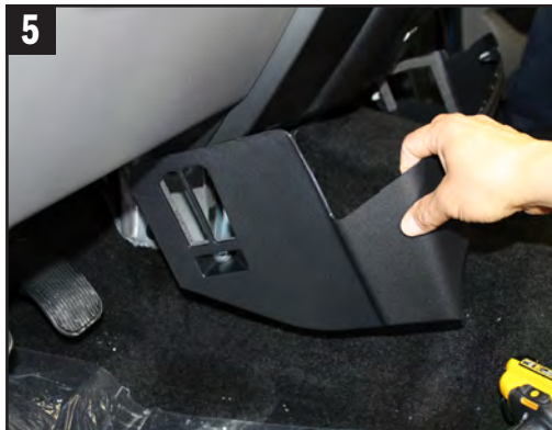
5. Remove (1) 10 mm screw holding the lower trim in place rotate over the transmission hump and unsnap from the passenger side.
