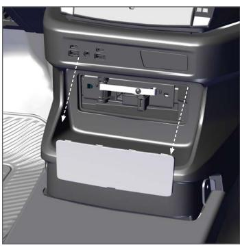
Remove the trim exposing the Manual Park Release (MPR). With the trim removed and Console installed, this will make access easier by only removing one Console Faceplate/Radio.
