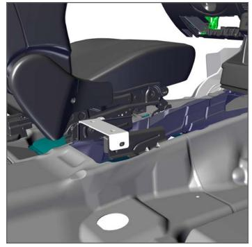
Attach the Console Mount Bracket with previously removed OEM hardware to the rear OEM Floor Plate mounting points.
