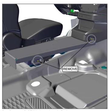
Remove (4) OEM bolts and retain for later use. Set OEM Floor Plate aside.
