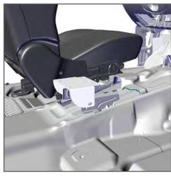
Attach the Rear Console Mount Bracket with previously removed OEM hardware to the rear OEM Floor Plate mounting points.
