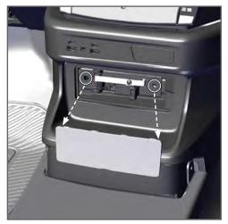
Pop loose the trim and remove exposed hardware securing the Manual Park Release (MPR) to the lower Dash Structure.
