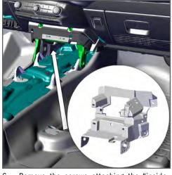
Remove the screws attaching the "inside lower trim structure" from the dash. Set Aside.
