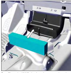
. Place the HVAC plug into the center air outlet.
