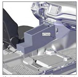
10. Attach the lower front Driver Side and Passenger Side of the Console with previously removed OEM hardware.
