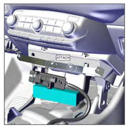
Attach the Front Console Mount Bracket with (2) existing OEM dash screws.
