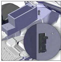
11. Attach the Manual Park Release (MPR) the side of the Console with provided hardware.
