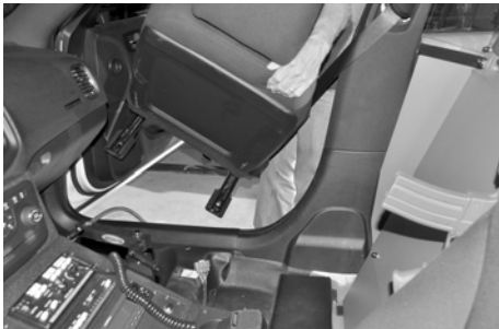
Remove both driver and passenger side front seats using E14 socket. Set seats aside.
